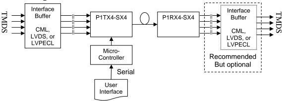
The input to the P1TX4A-SX4-01 must be AC-coupled. The output from the P1RX4A-SX4-01 is CML.
